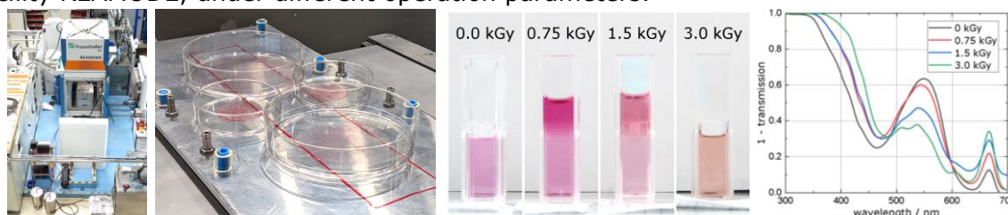
Figure 1. Experimental setup (left) and radiochromic effect of liquid roselle dosimeter (right)
