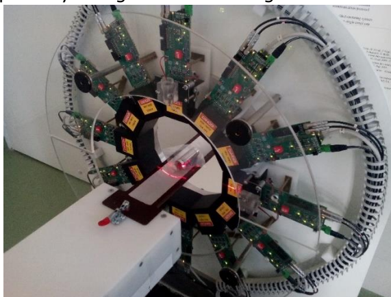
Figure 1. ATOMKI Mini-PET with the irradiated machine part
