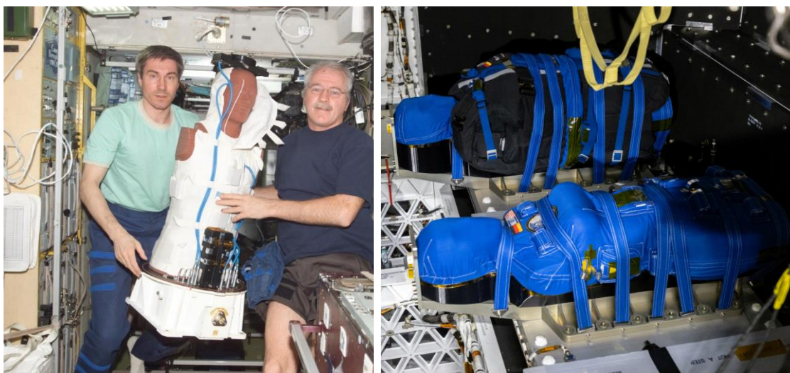
Figure 1. Left – astronauts unpacking the Matroshka phantom at the ISS to dismount TLDs; Right – two phantoms with TLDs inside in the Orion spacecraft before the launch of Artemis I
